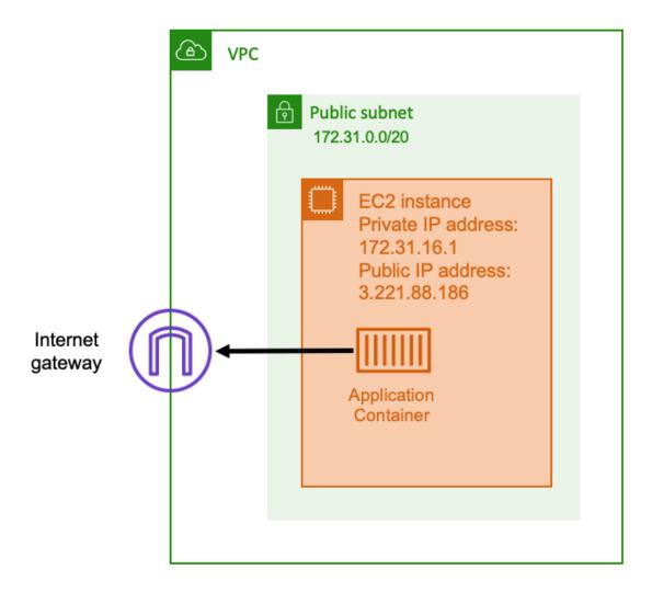
Using a public subnet that has a route to an internet gateway, your containerized application runs on a host inside a VPC on a public subnet. The host that is running your container is assigned a public IP address which is routable from the Internet. For more information, see Internet gateways in the Amazon VPC User Guide.
