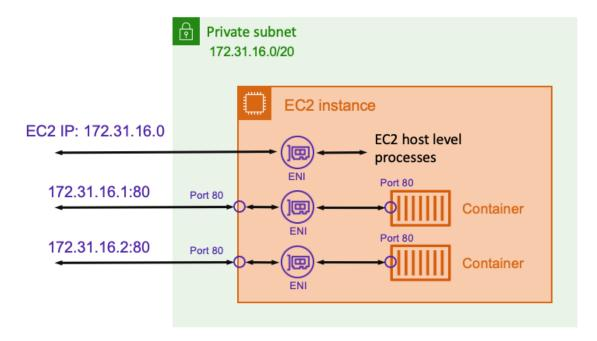
In the example above, the Amazon EC2 instance has its own ENI, which represents that EC2 instance's IP address that is used for network communications at the host level. Each task has its own ENI as well, and its own private IP address. Because each ENI is separate, each container can bind to port 80 on the task ENI. Rather than having to keep track of port numbers, you can send traffic to port 80 at the IP address of the task ENI.
