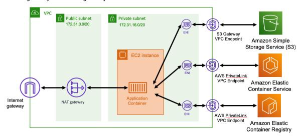
The following are some of the common VPC endpoints that are used with the Amazon ECS service.
