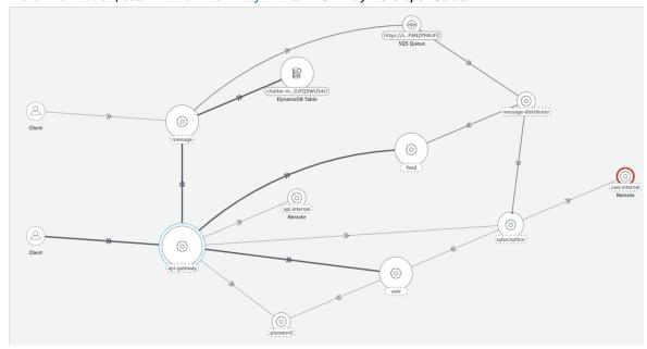
You can also explore graphs of how your services network with each other, and explore aggregate stats about how each service to service link is performing. You can also dive deeper into a specific transaction to see segments representing network calls associated with that particular transaction.
