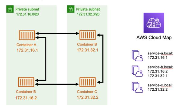
In the diagram above there are three services. serviceA has one container and needs to talk to serviceB that has two containers. serviceB needs to talk to serviceC which has one container. Each container in these services are able to use the internal DNS names from AWS Cloud Map to find the internal IP addresses of a container from the downstream service that it needs to communicate to.
