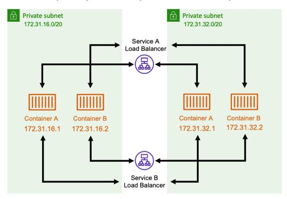
The load balancer maintains high availability by deploying redundant resources into each subnet. When a container from serviceA wants to talk to a container from serviceB it opens a connection to the load balancer. The load balancer then opens a connection to a container from service B. The load balancer serves as a centralized place for managing all connections between each service.
