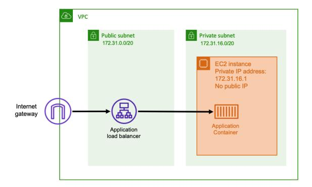
With this architecture, you create an Application Load Balancer in a public subnet so that it has a public IP address and can receive inbound connections from the Internet. When the Application Load Balancer receives an inbound connection and sees an HTTP request, it will open a connection to the application using its private IP address and forwards the request over the internal connection.
