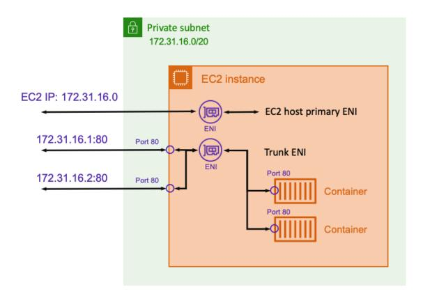
When using ENI trunking, two ENI attachments are consumed by default. The first is the primary ENI of the instance, which is used for any host level processes. The second is the trunk ENI which Amazon ECS creates. This feature is only supported on specific Amazon EC2 instance types.
