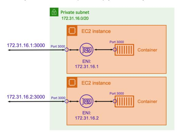
Using the example above, imagine you are running a Node.js container with an Express application that listens on port 3000. When the host network mode is used, the container receives traffic on port 3000 using the IP address of the underlying host Amazon EC2 instance. There is no mapping or virtual network. Instead, the container ports are mapped directly to the same ports on the Elastic Network Interface (ENI) attached to the underlying Amazon EC2 instance.
