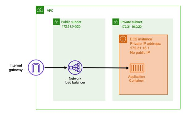
A Network Load Balancer as an ingress is very similar to an Application Load Balancer in that it is created in a public subnet, so that it can have a public IP address that is reachable from the Internet. The Network Load Balancer then opens a connection to the private IP address of the host running your container, and sends the packets from the public side to the private side.
