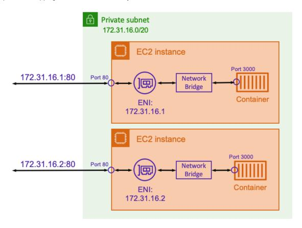
With a static port mapping, you explicitly define which host port you want to map to a container port. Using the example above, port 80 on the host is being mapped to port 3000 on the container. To communicate to the containerized application, you send traffic to port 80 to the Amazon EC2 instance's IP address. From the containerized application's perspective it sees that inbound traffic on port 3000.
