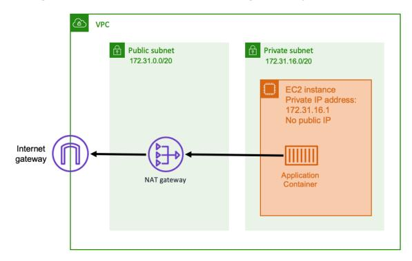
Using a private subnet and a NAT gateway, your containerized application runs on a host that is in a private subnet. The host has a private IP address that is routable inside your VPC, but isn't routable from the Internet. This means that other hosts inside the VPC can make connections to the host using its private IP address, but other hosts on the internet can not make any inbound communications to the host.
